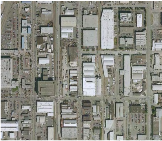
Figure X. An industrial area in Seattle, Washington where rooftops cover the vast majority of the site with paved roads consuming the rest.
